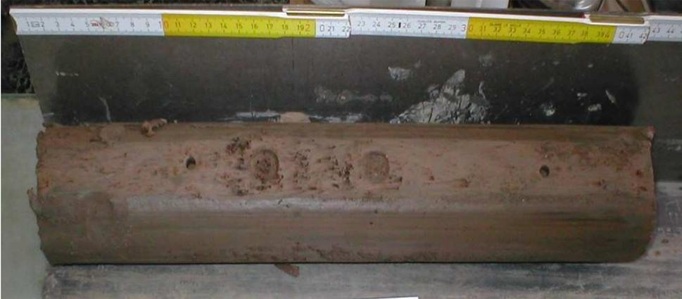
Pocket penetrometer (Kg/cm<sup>2</sup>) = **1,2** (kPa) **117,7**
