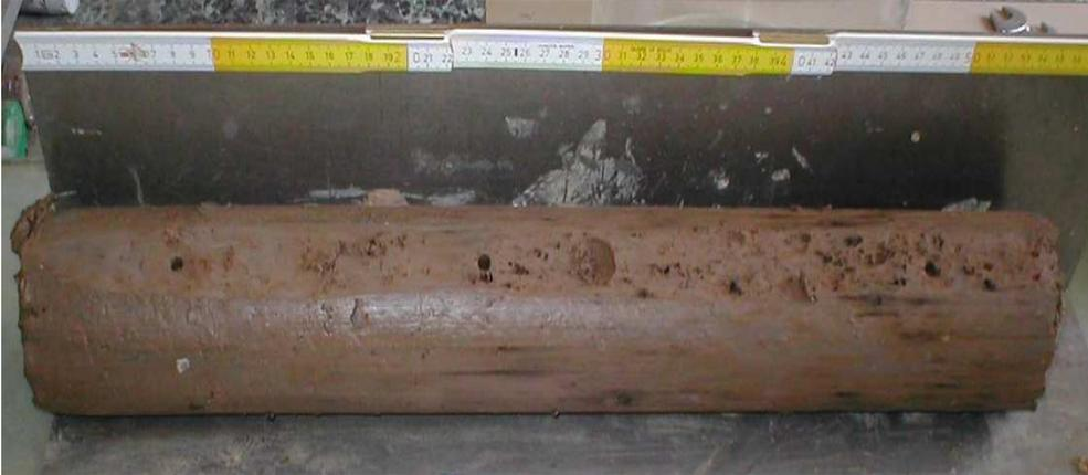
Pocket penetrometer (Kg/cm<sup>2</sup>) = **1,6** (kPa) **156,9**
